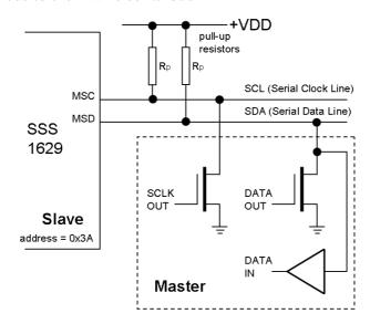
Bit transfer on the SSS1629 2 wire serial bus
