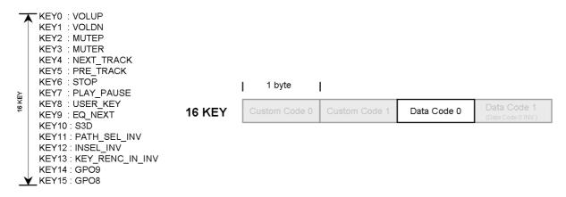
In 16 Key mode, *Data Code 0* can be set by user definition, and *Data Code 1* will be automatically inverted according to the *Data Code 0* setting
