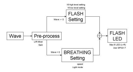
When setting for audio output indicator, it can be adjusted in accordance with the desired output range; each indicator signals can have 16 levels to do proposed audio settings.
