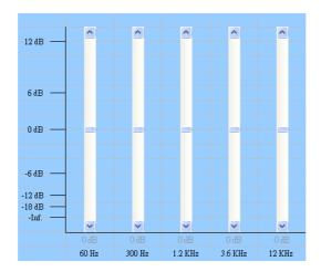
User can adjust a variety of sound effects according to requirement; the results will be stored in EEPROM after adjustment, and it can use single button to change different sound effect in cycle approach, simultaneously, also provide a single LED for indication of ON/OFF sound effect. By default, SSS1629A4 built-in a subwoofer sound settings, therefore, under no external EEPROM case, there is still an EQ sound transformation for user. Preset bass (SUBWOOFER) sound settings are as follows:
